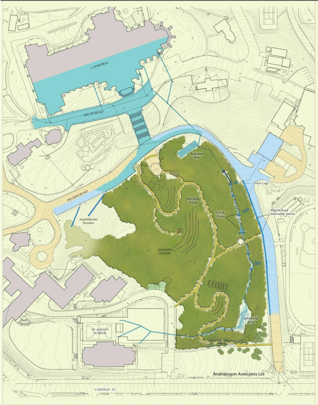
Figure E2: Washington National Cathedral Olmsted Woods and All Hallows Amphitheater restoration project to correct stormwater erosion using stone gutters, collection systems and infiltration to groundwater. (Andropogon Associates and Michael Vergason Landscape Architects)
